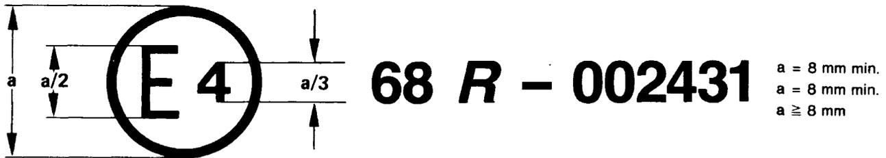
The above approval mark affixed to a vehicle shows that the vehicle type concerned has been approved in the Netherlands (E 4) with regard to the measurement of the maximum speed of motor vehicles, pursuant to Regulation No. 68 and under the approval number 002431. The first two digits of the approval number indicate that the approval was granted in accordance with the requirements of Regulation No. 68 in its original form.
